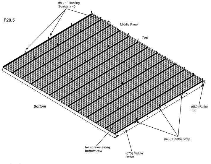
DO NOT overtighten screws, could cause damage to roofing material
