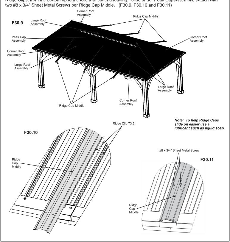
Components 12 x #8 x 3/4" Sheet Metal Screw 6 x Ridge Cap Middle
