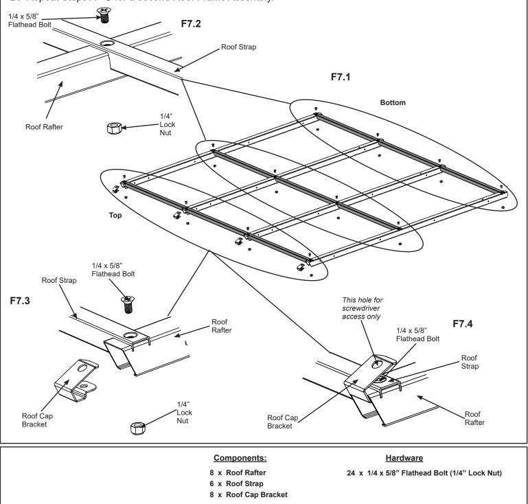
**D:** Repeat Steps A - C for a second Roof Frame Assembly.
