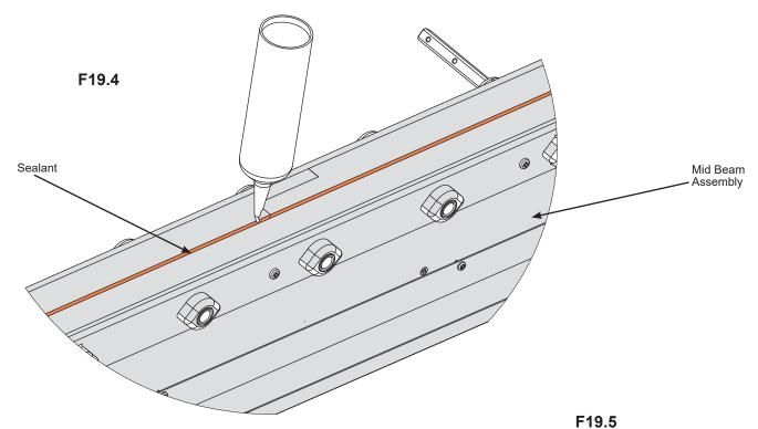
**Note:** All surfaces to be clean, dry, dust and grease free before application with temperatures above 5°C (41°F), no warmer than 35°C (95°F).
