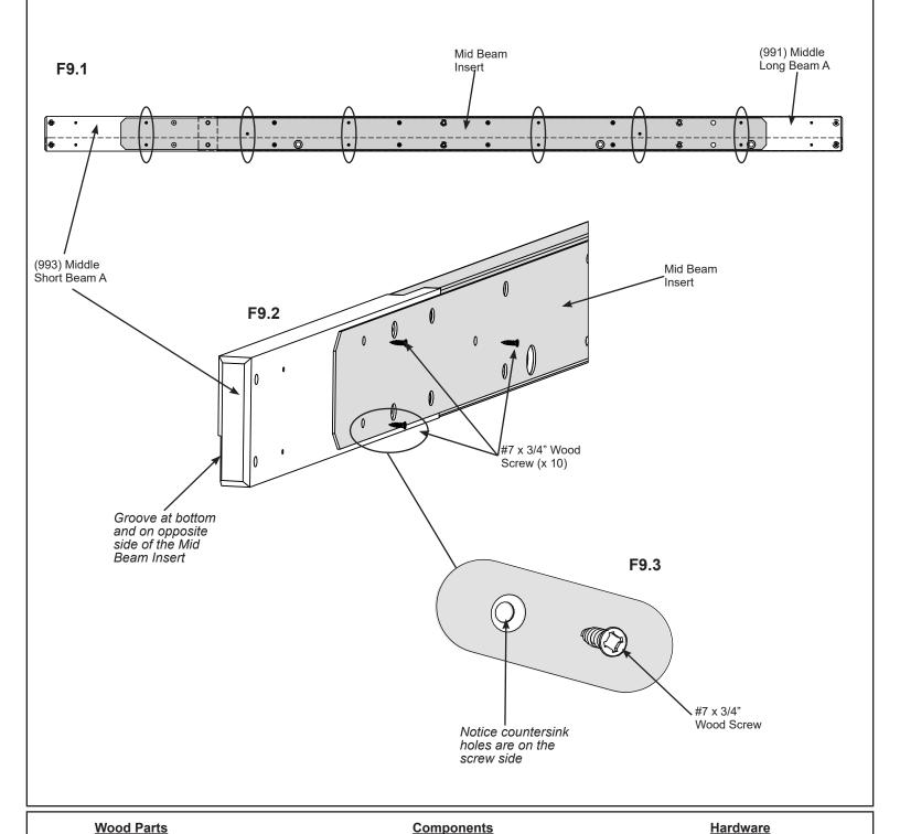
1 x (991) Middle Long Beam A 1 x (993) Middle Short Beam A 1 x Mid Beam Insert
