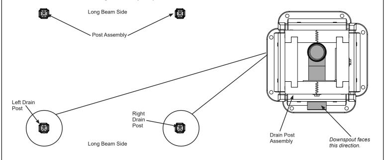
Option 2 shows the drains downspout exiting on opposite Short Beam sides.
